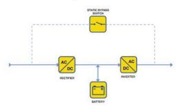
This AC->DC->AC function allows for two big advantages over other UPS technologies.
